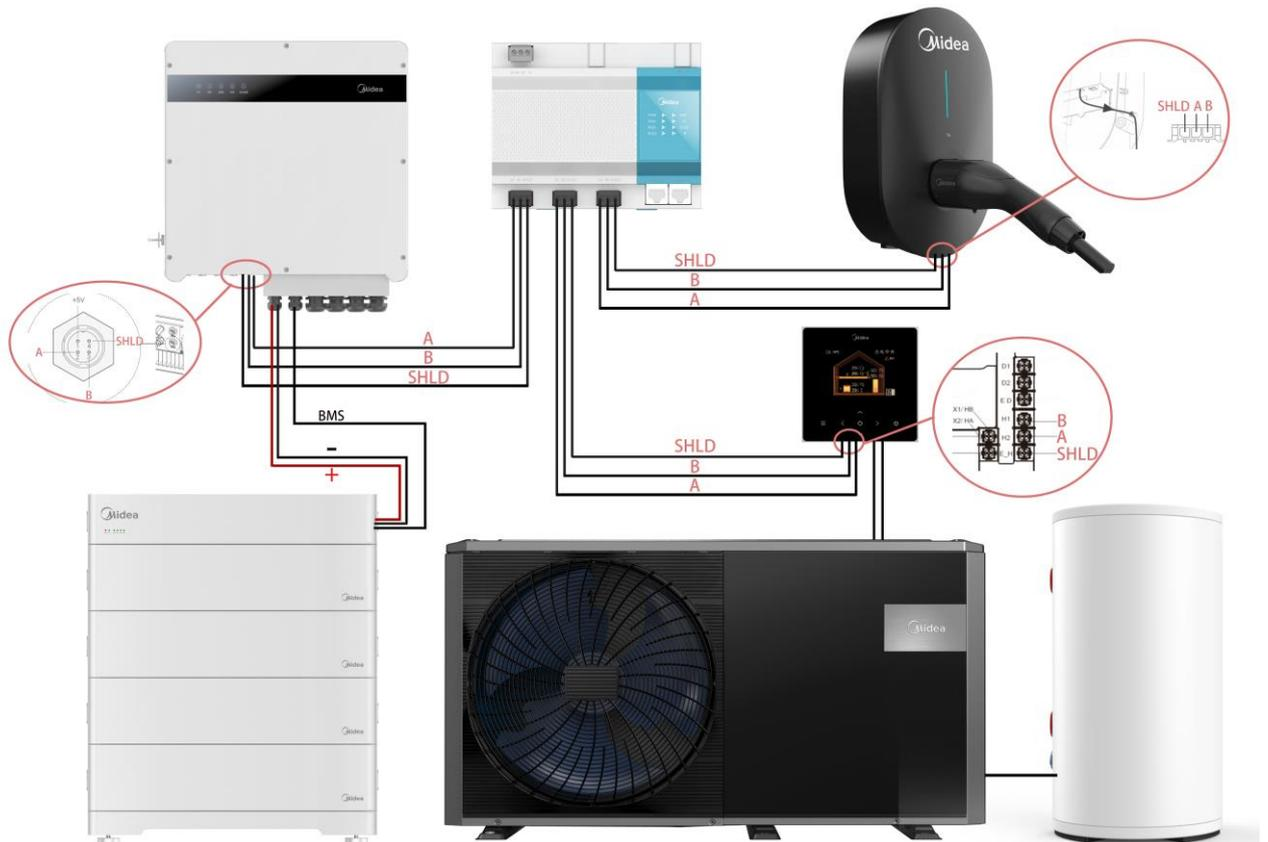
The wiring amplification diagram is shown below:
